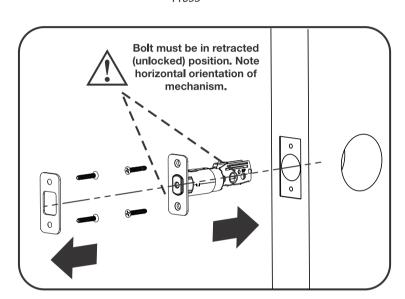
2 Installing Keypad Escutcheon
