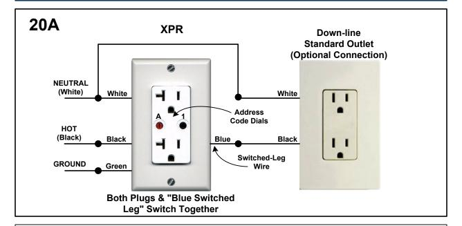
**Description:** The XPR, 20A Duplex Receptacle is used as a Remote Load Switching Module, which responds to X10 ON/OFF Commands from an X10 PRO Controller. Loads may be plugged into either one of the top/bottom receptacles or hard-wired from the Blue Switched Leg Wire to external loads or down-line receptacles.
