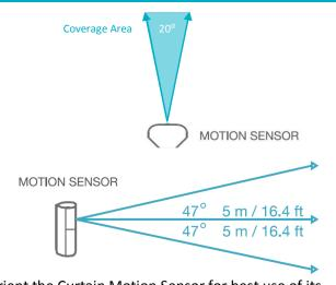
Orient the Curtain Motion Sensor for best use of its detection zones.
