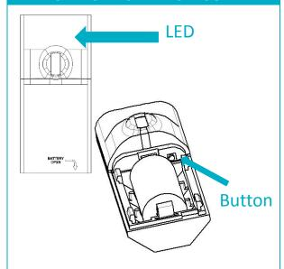
Test the Curtain Motion Sensor from the desired location before permanently installing it by pressing the button twice to check network status.
