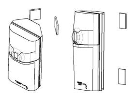
Install the Curtain Motion Sensor on a clean surface using the 2-sided tape provided. It can be installed on a flat surface or in a corner, vertically, horizontally or upside down.
