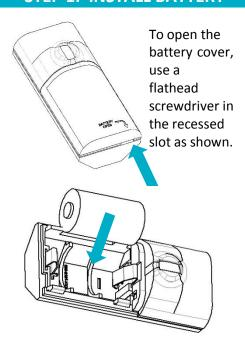
Remove the packing tape, if present, from the battery cover and install the CR2 battery with polarity as shown.
