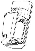
Verify that the device is sensing motion. The sensor requires a 3 minute "warm-up" time before it will report motion. The LED should flash red and motion should be indicated on your web portal or smart phone application.
