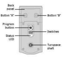
Note: When the cover is removed, the tumpiece shaft can be used to manually lock and unlock the door,
