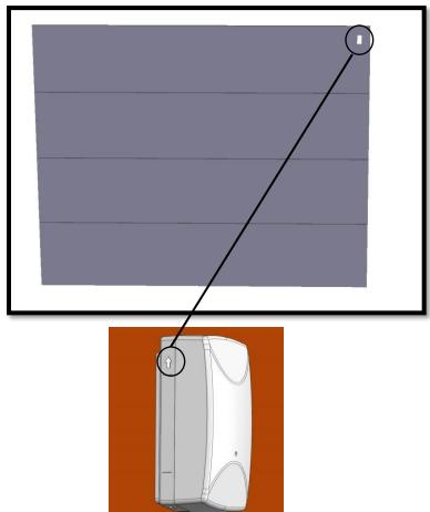
IMPORTANT: The Tilt sensor must be located on the top panel AND have the arrow on the side of the sensor pointing UP in order to operate
