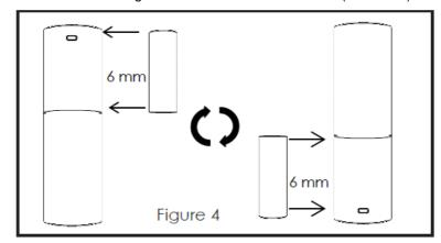
For optimal performance, it is highly recommended to install the Door/Window sensor on the fixed frame and the magnet on the moving part of the door/window, rotate if necessary. Place the sensor near the top of the door that close to the opening edge of the door. This is the mounting location for the sensor.
