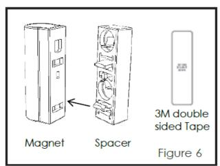
4. Use provided double-sided tape on the magnet. Make sure the alignment of both sensor and magnet is correct. The magnet aligns from the top of the sensor case near the button and LED. Press firmly and hold in place for a few seconds. If the spacer is used, it can be mounted to the door using screws and/or double-sided tape before attaching the magnet. Secure tape-mounted parts with silicone if needed.
