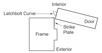
Curve of latchbolt must contact strike plate first.
