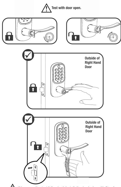
If key operation test fails, check installation beginning with Step 6.
