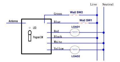
For "Inclusion" in (adding to) a network: Put the Z-Wave<sup>™</sup> Interface Controller into "inclusion" mode, and following its instruction to add the ZL 7432 to your controller. To get in the "inclusion" mode, the distance between module and controller is suggested to be in one meter. Turn on and turn off the wall switch that connects with ZL 7432 module 4 times to be included. (or press the Program SW 4 times within 2 seconds to be included)
