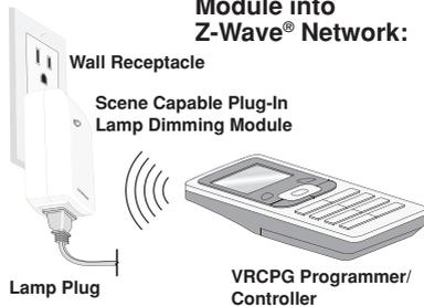
**NOTE:** Programmer/Controller must be in close proximity to Scene Capable Plug-In Lamp Dimming Module when including into network
