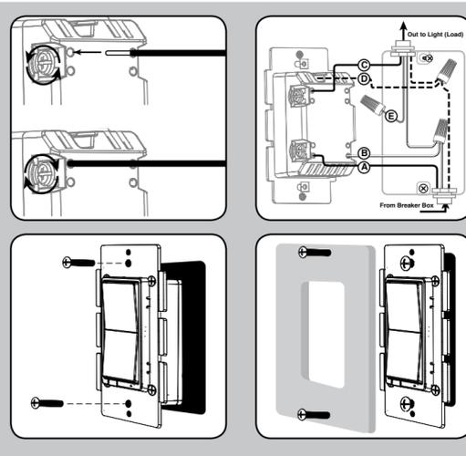
**Note: The Traveler terminal is only used for 3-way or 4-way wiring and should remain insulated if the switch is being installed in a 2-way system (one switch & one load).**
