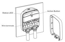
Action button: Used for Heavy Duty Smart Switch's Z-Wave network inclusion and exclusion and to manually turn on/off;
